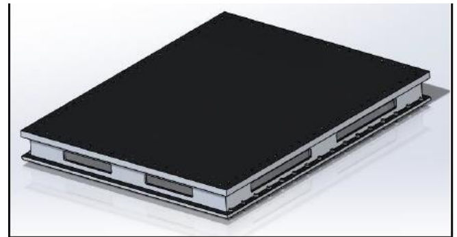
Figure 5: Fixture used for vibration Testing, 90 inches by 60 inches
